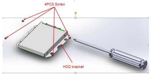
Step 2: Install the dampers in the bracket and fix by four screws.
