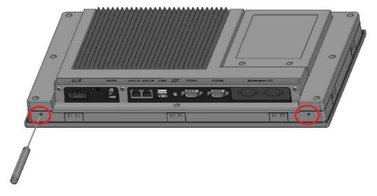
**Step 3**: Set TPC cross the cut-out hole and push it into the wall, the snap hook will hold the machine on the wall.
