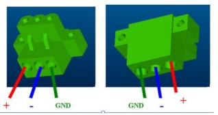
**Figure 2.2 Pin Definition of Power Connector**
