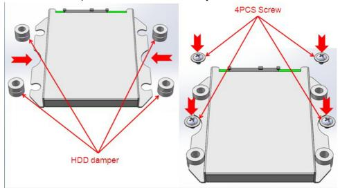
Step 3: Install HDD module into system and then cover back the side cover to finish.
